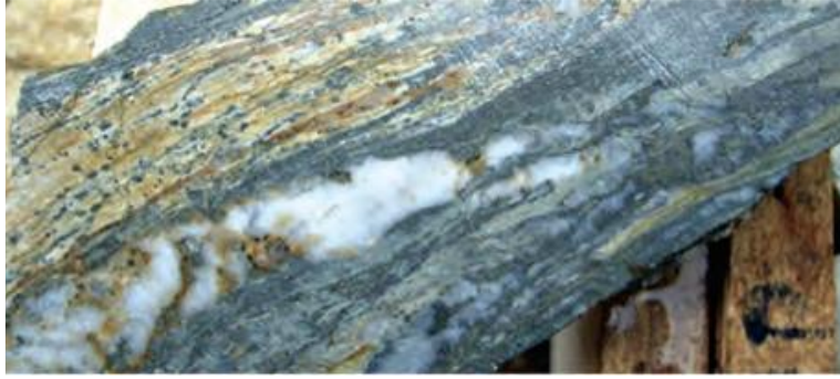
Figure 3 - Quartz and pyrite in albitised syenite overprinted by a shear fabric GKP 11.
