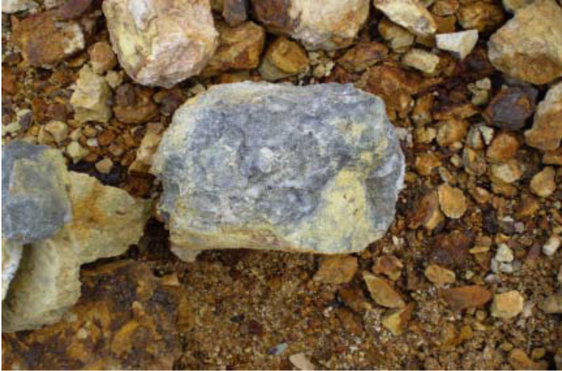
Figure 8: Example of quartz pyrite veining from Üzümlü workings
