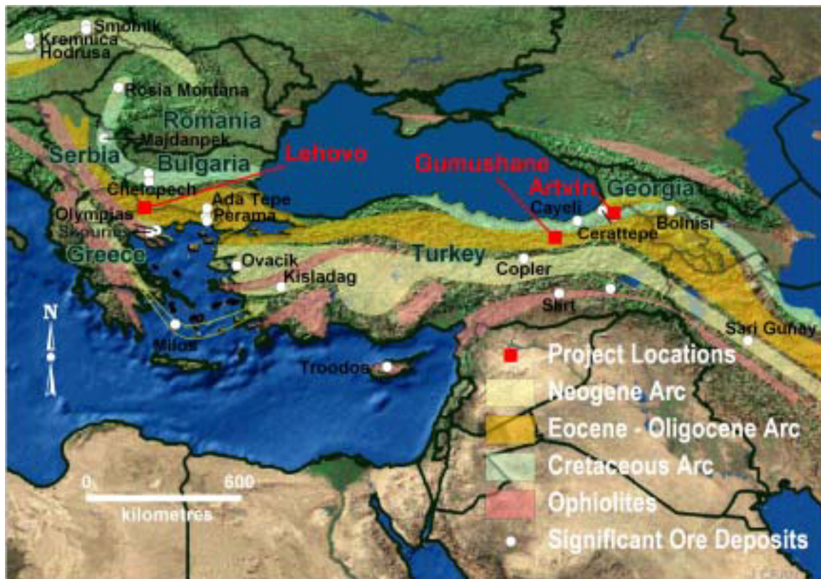
Figure 3: Location map of the project areas, regional metallogenic belts and significant ore deposits
