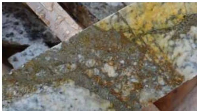
Examples of Mineralised Tula Kapi Drill Core
