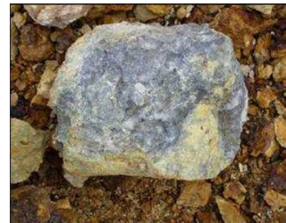
Example of quartz pyrite veining from Üzümlü workings
