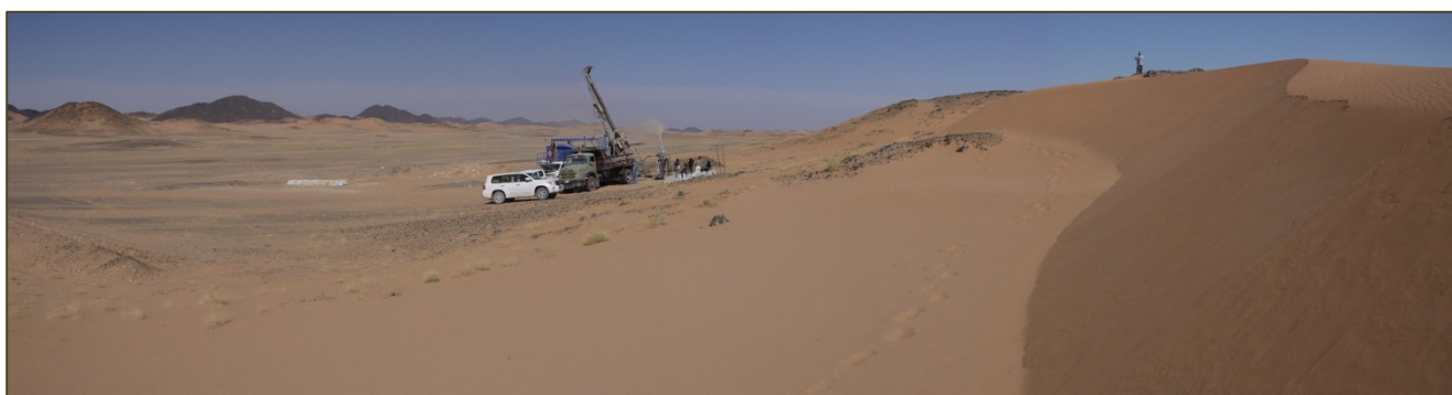
Reverse circulation drilling at Jibal Qutman East Zone Prospect
