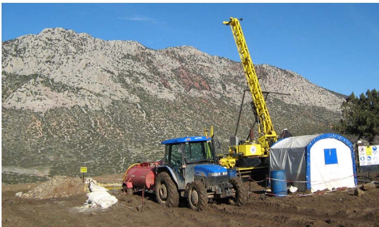
Diamond drilling at the Bakir Tepe Project, Turkey
